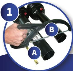
Remove guard and separate driveline halves. Shorten guard halves, pic. 1) and profile tube halves pic. 2) to required length.
