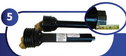
Reassemble guard halves. Both profile tubes should extend 40-mm (1.58") beyond the end of the guard tubes.
